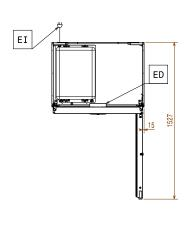
**Electric** Supply voltage: 220-240 V/1 ph/50 Hz Electrical power, max: 0.45 kW Capacity: Number and type of grids (included): 5 - 530x700 **Key Information:** Net Volume: 510 It Door hinges: External dimensions, Width: 900 mm 700 mm External dimensions, Depth: External dimensions, Depth with 1527 mm Doors Open: External dimensions, Height: 2040 mm Number and type of doors: 2x1/2 Full 772 mm
